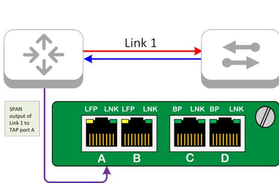
Diagram 1: SPAN port sends a mirrored output
