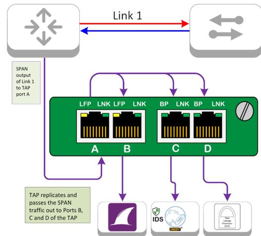
Diagram 2: SPAN mirrored output regenerates traffic to send to appliances
